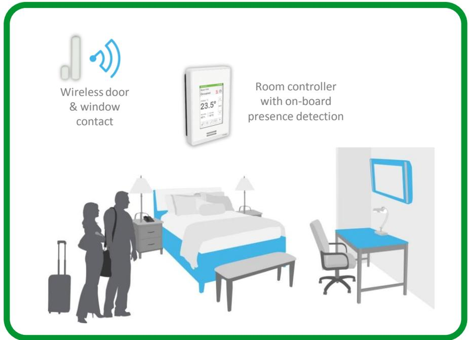
As these systems continue to evolve, use of advanced presence detection approaches are now merging with the concept of “target” temperature settings to manage activation of heating and cooling systems in guestrooms. These settings allow the room temperature to fluctuate up or down a pre-determined temperature range. Hotel operator-selected variances, setback, and deep setback settings help to keep the room at desired temperature ranges throughout various room status scenarios.
